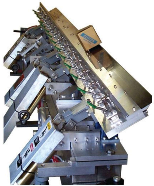
FIGURE 1. A doctor blade system featuring on-press blade change capability without the use of tools or clamping bolts
